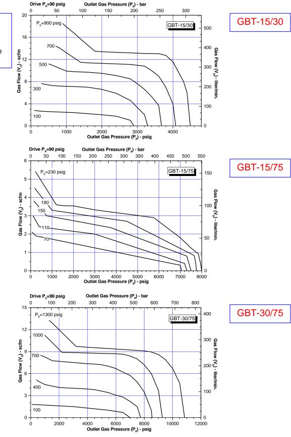
Legend PA = Drive Pressure PO = Gas Outlet Pressure PS = Gas Inlet Pressure VO = Output Gas Flow
